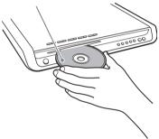
To load other discs, press DISC1-5  $\triangleq$  (that is not loaded a disc) and load the disc after "NO DISC" appears in the front panel display.
